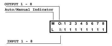
If no audio is being fed to the unit on any channel the numbers in the lower half of the display will be inverted indicating no audio present. After 5 seconds of audio application on a given channel above threshold the respective lower channel indicator will become un-inverted indicating audio present above the on the channel.
