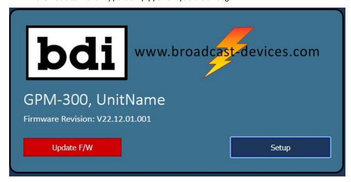
2. Press setup. DO NOT PRESS UPDATE! Doing so will do no harm but you will lose access to the unit and the unit will need to be power cycled. This button is only used for updates in firmware provided by the factory.
